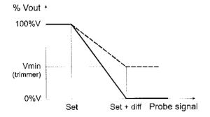
If the input signal is lower than the Set, the output signal is 230 Volt (fans are running at the maximum speed). When the signal increases and enters the range between the Set and Set+Diff the output signal follows the temperature variation. Above the Set+diff value the output signal is always 0 Volt (if no Vmin has been set).
