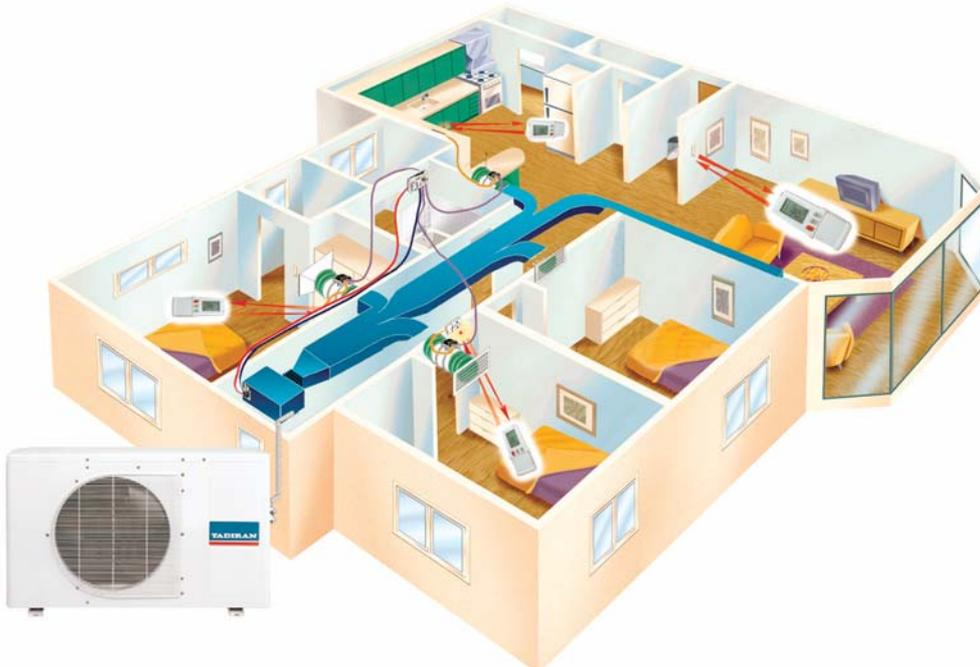
A multiple zone air conditioning system. It allows you individual room/office comfort by integrating the various temperature requirements of each room, notifying the main controller and operating a 5-step-damper system in each room.
