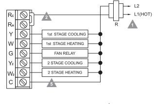
Wiring-conventinal system: 1 transformer
